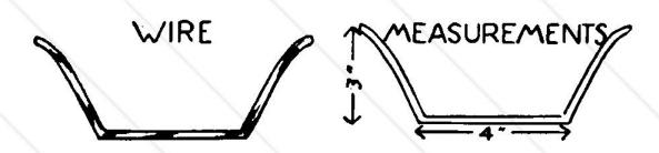
ture of the object; twice this distance plus the diameter of the base equals the amount of metal required. If a perfect spherical shape is to be formed, cut the metal about an inch larger than the desired size.
